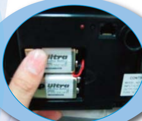
Figure 6: Install the 9 volt batteries
