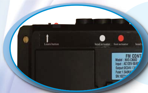
Figure 2: The red LED will light up when the control box is in the learning mode.
