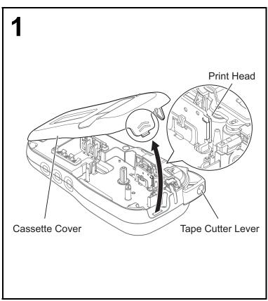
With the LCD facing down, open the Cassette Cover by pressing the grooved tab and pushing the cover in the direction of the arrow, as illustrated.
