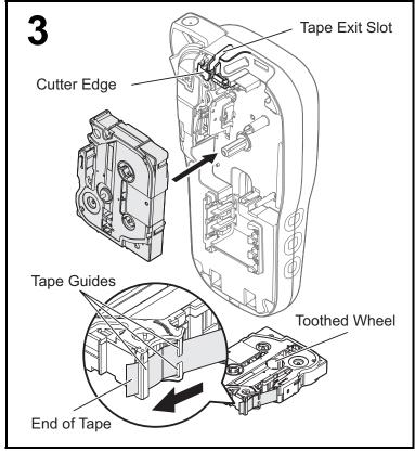
Insert the Tape Cassette following the drawing marked inside the case. Gently press the Cassette into the P-touch labeling system until it locks into place.
