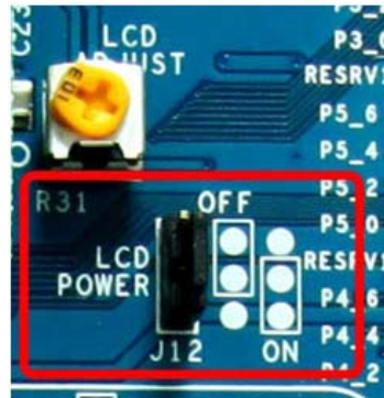
Figure 5-28. CY8CKIT-001 PSoC DVK LCD Power Jumper
