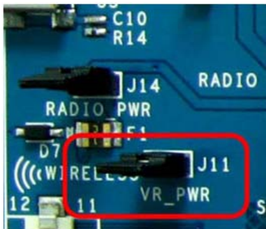
Figure 5-29. CY8CKIT-001 PSoC DVK VR_POWER Jumper
