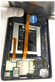
Remove cross-head screws from LCD BTB Fix STEEL.
