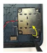
Separate the 2 Speaker BOX and cables from Furnished Middle Casing.
