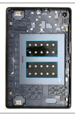
② Stick the new battery adhesive onto the Furnished middle casing according to the positioning line. Ensure it is firmly attached.
