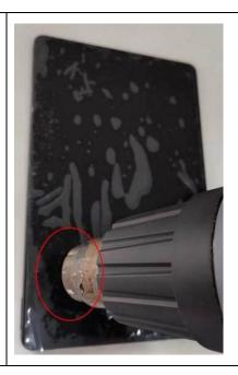
Pull up on the suction cup at USB side to separate the LCD + Touch Panel from enclosure. Insert a Plastic Plectrum in the gap between the LCD + Touch Panel and Furnished Middle Casing.
