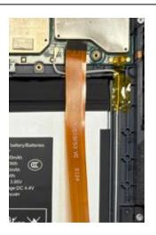
Put the Furnished Middle Casing on a heater at 75°C with the battery facing up and heat for 5 minutes.
