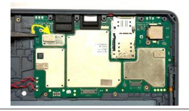
PCBA (with speaker box) removal completed. Remove the Camera. Remove the front camera. Remove the Speaker BOX -R and Speaker BOX-left with a Solder iron.
