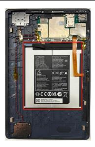
There are battery adhesives between the battery and Furnished Middle Casing. Insert the plastic scraper along the gap to separate the battery.
