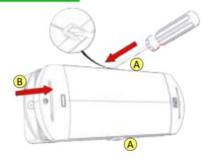
To dismantle the luminaire, simply remove the difussor.
