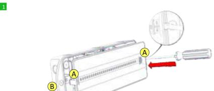
Place a flat blade screwdriver to the recesses (A) and pull up gently the reflector (B) to remove it.
