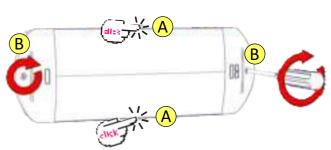
The plastic latches (A) must be secured (click sound). Fasten the 2 screws (B). (Tightening torque 1.2N\*m)
