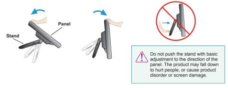
2 After adjusting the angle of the panel for convenience, lock with the locking handle to prevent the product from moving.
