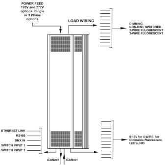
iCANnet cable type – Cooper LCCNP (Non Plenum) Cable or LCCP (Plenum) or Belden 1502R (Non Plenum) or 1502P (Plenum).
