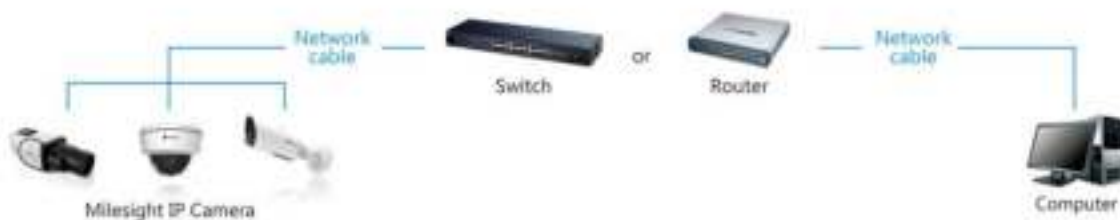
Figure 2-1-2 Connect via a switch or a Router
