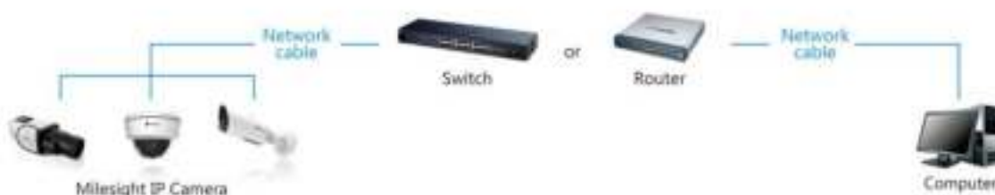
Figure 2-1-2 Connect via a switch or a Router
