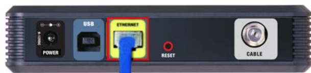
Back view of cable modem
