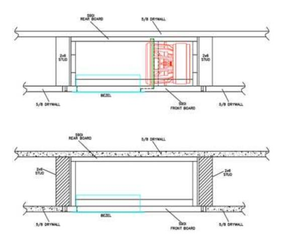
The front board of the S90 is made from 5/8" MDO plywood, which presents a smooth, paintable finish surface similar to dry wall. It can be butted up against the 5/8" dry wall, taped, and spackled, and painted like any other section of wall. It will also readily accept skim-coating if the construction calls for plaster walls.
