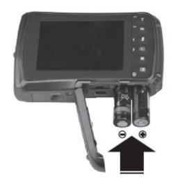
Insert 2 x AAA (1.5V) batteries. Alkaline batteries recommended (not included).
