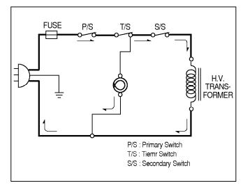
• 3.2 volts AC is generated from the filament winding of the high voltage transformer. This 3.2 volts is applied to the magnetron to heat the magnetron filament through two noise-preventing choke coils.
