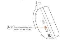
After using the headset with one device for more than 5 minutes, if you need to connect the headset to another device, you can clear the existing pairing information by pressing the PREV button four times consecutively (within 1.5 seconds). This will enter them into pairing mode for reconnection.
