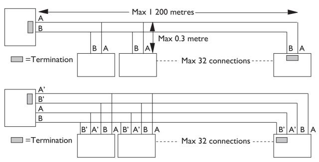
**N.B.** R+/R-, T+/T- definitions are not standard, it can help to shift A and B if the unit does not work.
