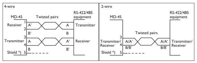
\*) If shielded cable is used, connect the shield only at one end to avoid ground currents.
