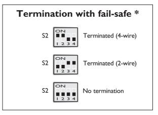
\* The fail-safe function forces the signal state of the receiver to OFF when the connected transmitter is in tri-state (transmitter inactive). The receiver located furthest away shall be terminated.
