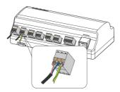
step 4 Connect the DC cable led from the "24V IN" port of the Logger1000 to the "DC 24V OUT" port of the power box. Connect the stripped AC cable to the "AC (100~277V)" port of the power box, and connect the other end of the AC cable to the 220V AC power.
