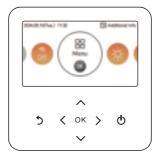
In the menu screen, press [<,> (left/right)] button to select the category to set, and press  $[\mathbf{OK}]$  button to move to the detail screen.
