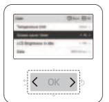
In each detail screen of the menu, as in the box in the left figure, when "<, >" icons are displayed at the same time, you can immediately apply the setting value by pressing [<, > (left/right)] button.
