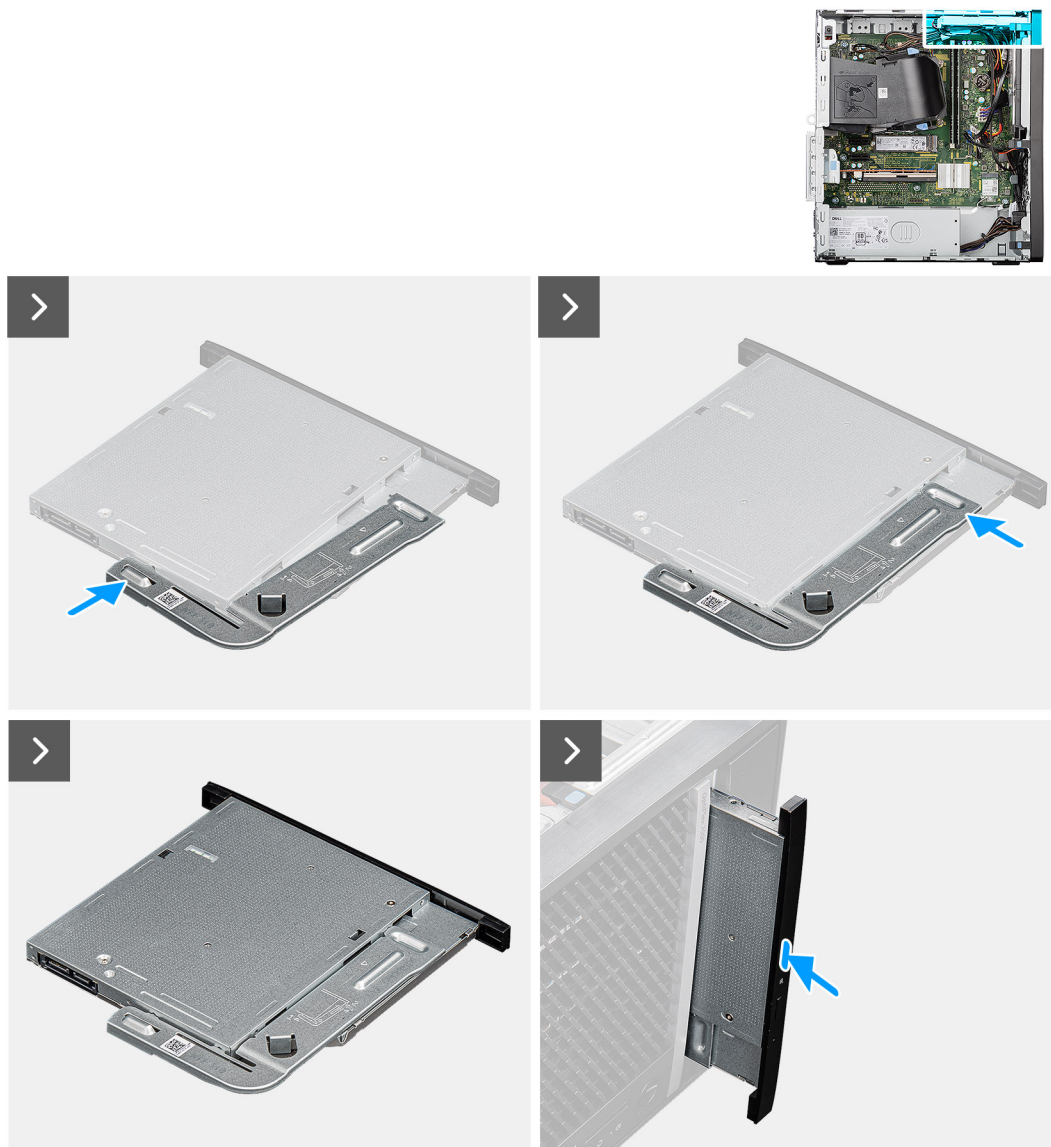
Figure 39. Installing the slim optical drive
