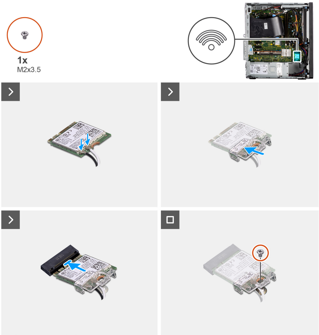
Figure 32. Installing the wireless card
