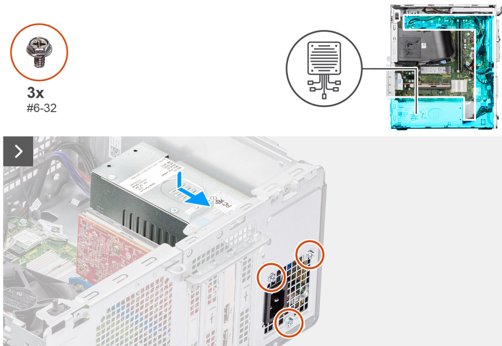
Figure 66. Installing the power-supply unit
