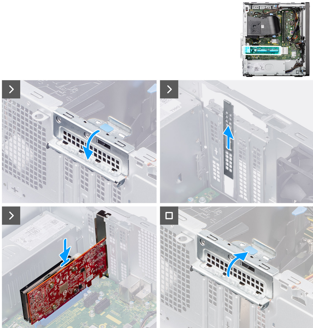
Figure 34. Installing the graphics card
