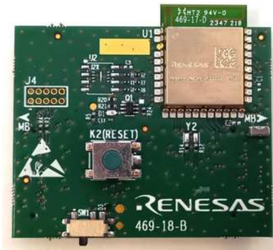
Figure 9. DA14592MOD module evaluation board
