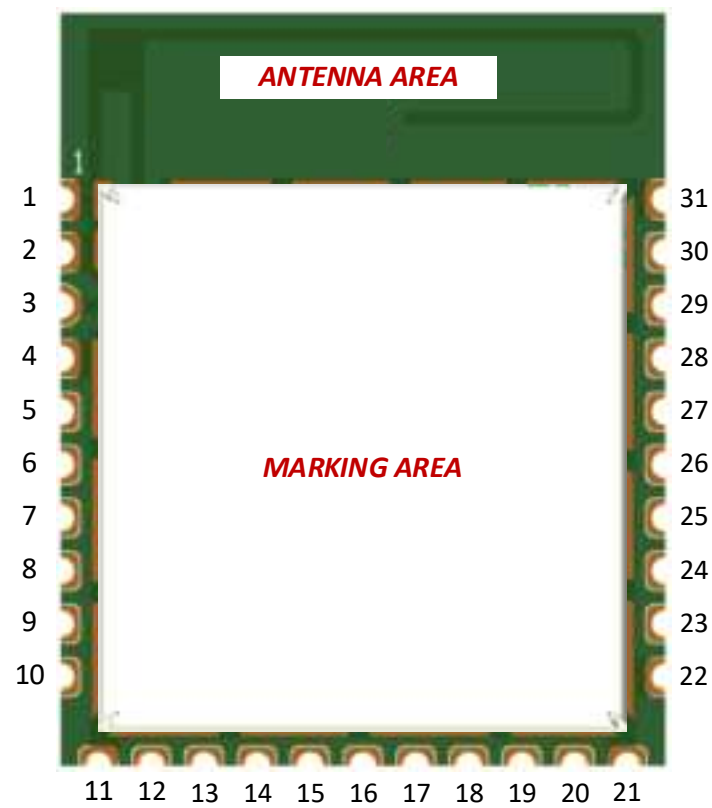
Figure 4. Pinout diagram – top view
