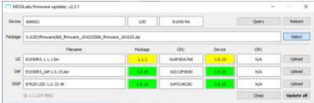
Figure 4.3: The firmware update tool shows the current versions of the firmware components, indicating which are up-to-date (green) and which require updating (yellow or red).
