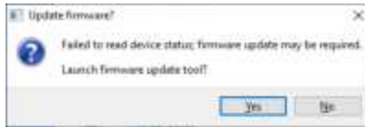
Figure 4.2: When mog1dd detects a version incompatibility it will offer to install a firmware update. Alternatively the Update option can be selected from the Help menu.
