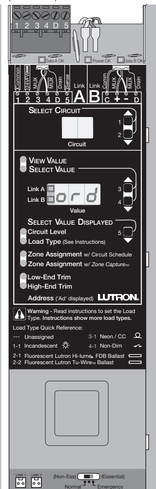
Circuit Selector in Emergency (Essential) Panel
