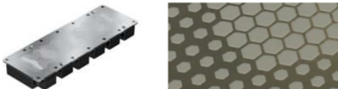
Figure 12: Application of PCM phase change material on SEMITRANS®10 baseplate and inhomogeneous honeycomb structure
