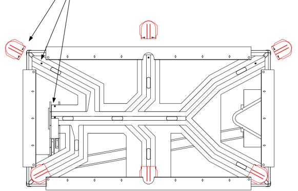
Step #5 - Remove The Four Die Cast Corners.
