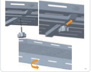
Adjust the basket to the suitable position. Tighten all bolts in the step 2.
