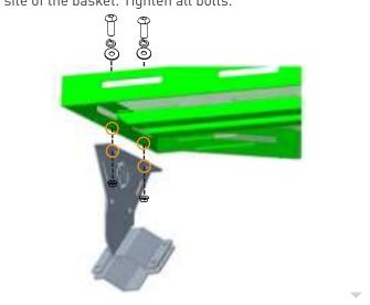
Install the plastic hand knobs to the basket. Slide the rail and open the basket when you use.
