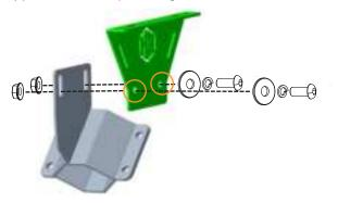
Assemble the top side brackets and the basket using (4) M6x16 button bolts, (4) split lock washers, (4) flat washers, (4) flange lock nuts. Repeat this step for the opposite of the basket. Tighten all bolts.
