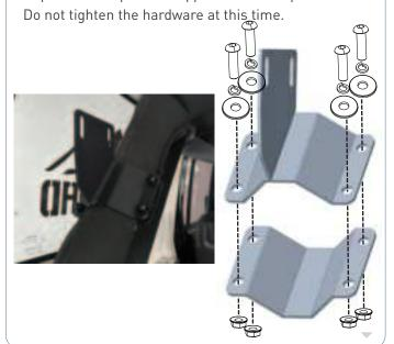
Install the top side brackets to the middle side brackets using (4) M8x20 button bolts, (4) split lock washers, (4) flat washers, (4) flange lock nuts. Repeat this step for the opposite of the c-pillar. Tighten all bolts.
