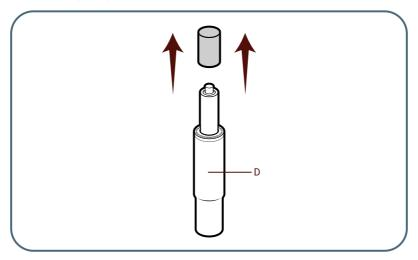
Turn the frame the right way round again and then put the chrome rosette over it. Then insert the gas spring (Part D) into the centre hole of the star base.
