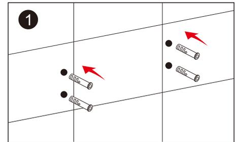
3. Knock 4 plastic expansion screws into the wall holes.
