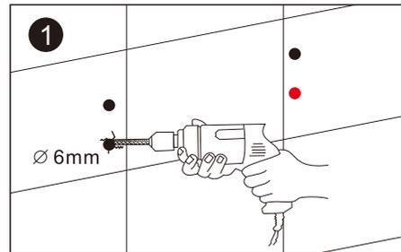
2. Drill holes in the marked positions with a 6mm drill bit.
