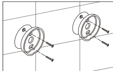
5. Use screwdriver tighten the mounting bracket on wall stable.
