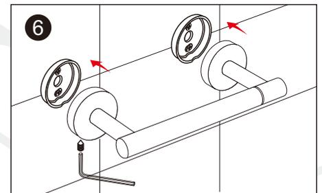
6. Put the base onto mounting bracket and tighten the setting screw in bottom.
