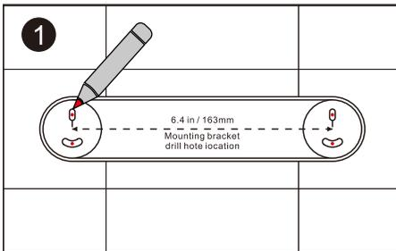
1. Press the "drill hole location card" horizontally on the wall, and mark the drilling position with a pencil.
