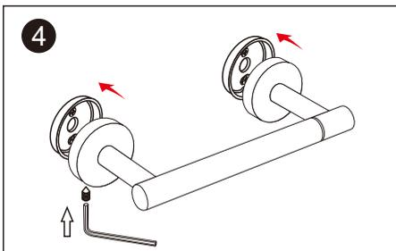
4. Loosen the fixed screw using the included allen wrench and remove the bracket cover from the base.
