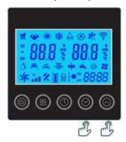
On the main interface, press and to adjust the desired water temp. of your pool, then press the to save the setting.
