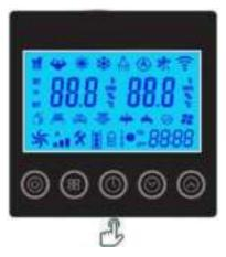
Press the button to enter the clock setting interface. Clock display on right bottom flashes.
