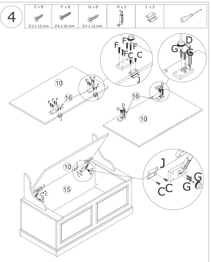
Fix two plate 16 to plate 10 using screw(F) as shown. Fix hinge(J) to plate 10 using screw(C) as shown. Fix part(D) to plate 16 using screw(G) as shown. Attach plate 10 to plate 15 by fix hinge using screw(C) as shown.
