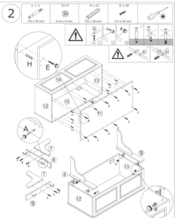
Cover plate 11 to the component with wooden dowel(H), then fix using screw(E) as shown.
