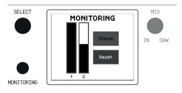
The MONITORING view screen is intended to be a visual representation of each of the volume levels for each of the direct monitoring signals. This Advanced Direct Monitoring functionality is quite unique as you can create a special direct monitoring mix, perfect for even the most special recording and monitoring situations. No matter if you record microphones or guitars or synthesizers, anything you need to monitor via your studio monitors or headphones can be setup directly on the hardware.
