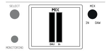
The MIX view that is displayed when you use the MIX encoder, shows a visual representation of the output/playback (DAW) and input (IN) signals.
