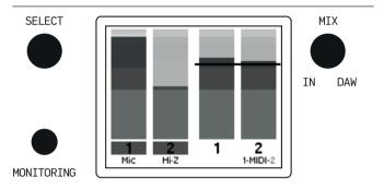
The standard view of the LCD screen shows the active signal levels for input channels 1 and 2 on the left half of the display area and the playback levels (DAW signal) for channels 1 and 2 on the right half of the display area as level meters. The level meters are separated into different colors. The red color on the top means that the signal is probably too loud and possibly clipping while an optimal signal level is typically orange. The green area indicates that a signal is present.
