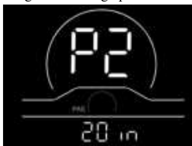
Fig. 4-2 Wheel Diameter Setting Interface
