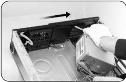
3 – Pull for ward the cable.
