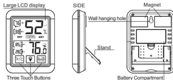
1. Display: Displays the current humidity and temperature, maximum and minimum humidity/temperature recorded in the past or past 24hrs.
