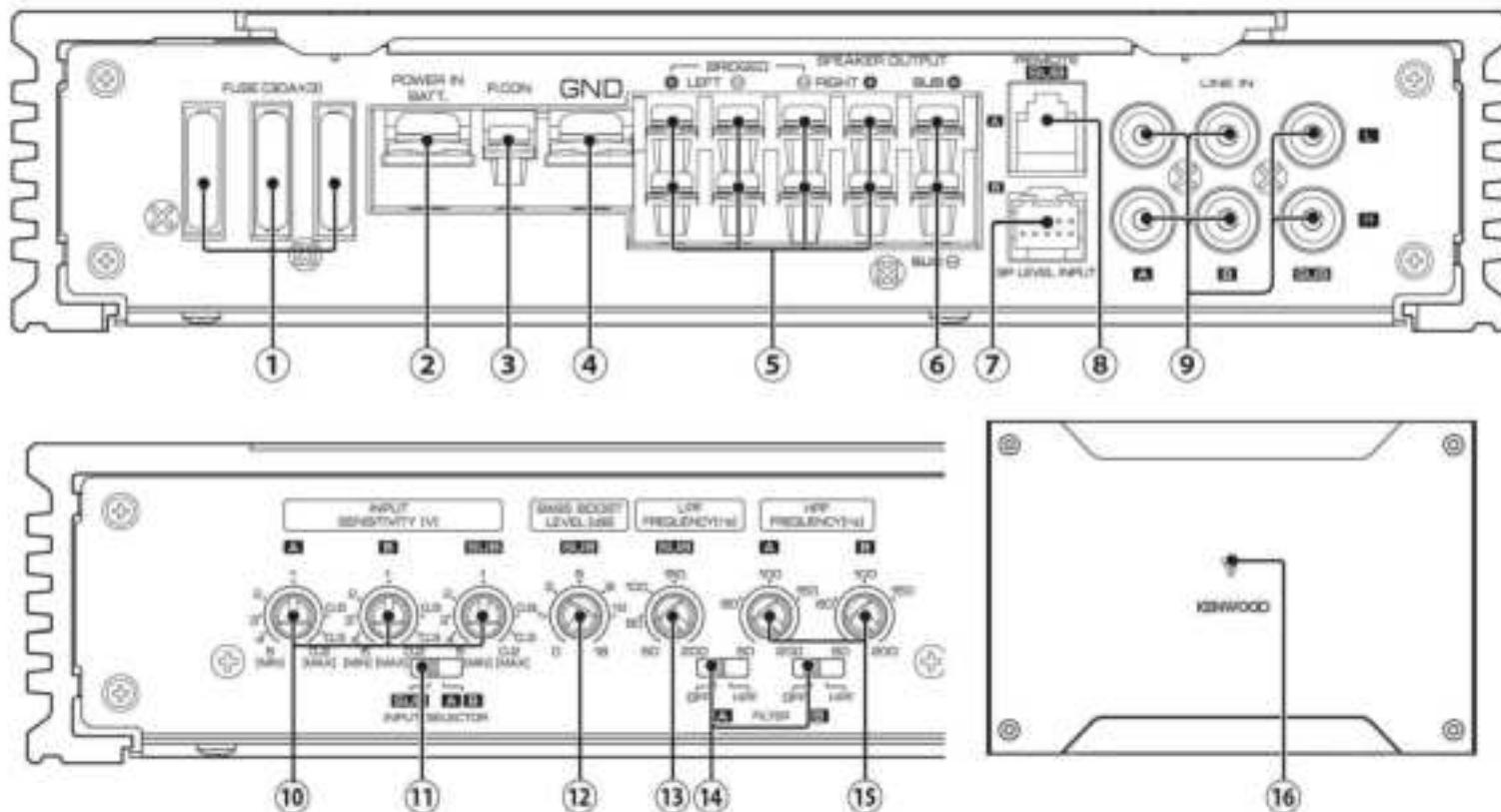
The unit is a 5-channel amplifier incorporating 2 stereo amplifiers and 1 monaural amplifier in a single body. The stereo amplifier on one side is called amplifier A, while the one on the other side is amplifier B. The monaural amplifier is called the amplifier SUB. This unit is compatible with a large variety of systems by combining the switches and functions described in the following.
