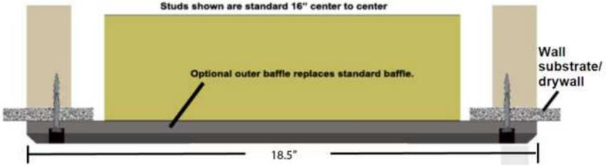
Pixel Pro can be ordered with an oversized outer baffle to allow for in-wall installation.
