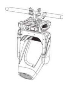
Step one: Installation the clamp onto the omega bracket;
