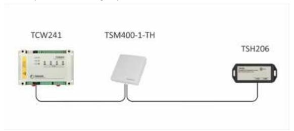
"Star" topology can be used only as a last resort for up to 4 sensors and a total cable length of up to 10 meters.
