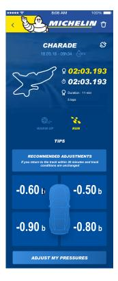
In Run mode, once you have pressed STOP, you will receive adjustment recommendations, you can access the pressure gauge function by selecting ADJUST MY PRESSURES.
