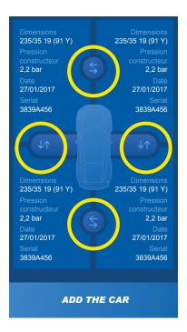
NOTE: Switching from front to rear is only possible for vehicles with exactly the same size tires on the front and rear.
