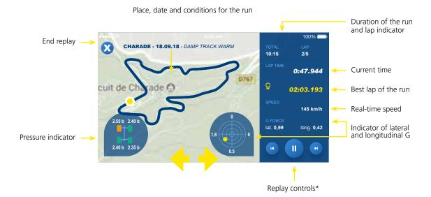
\*The Play / Pause functions are controlled by the same button. The arrows around the Play / Pause button are used to go from one lap to the next either backwards of forwards.
