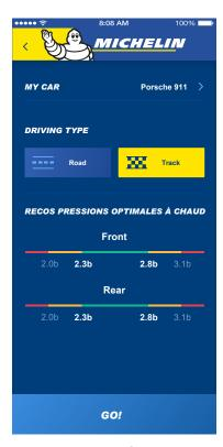
REMINDER: On-road, it is recommended to always check the pressure of your tires when they are «cold», meaning after driving less than 3 km (2 miles) at slow speed (in an urban area) or if the vehicle has been stopped for at least two hours. Otherwise, you must add 0.3 bars to your pressure. In on-road mode, the start of the green area for each of the axles corresponds to the pressure when cold recommended by the manufacturer.
