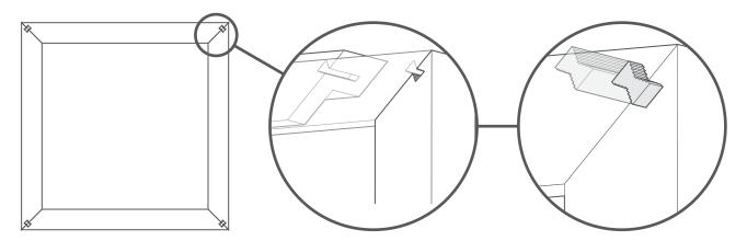
Line up all the corners, then insert the Hoffman keys from your fittings kit to join the frames securely together. The key can be a little tight, so you may have to give it a few taps with a hammer to fully insert it.
