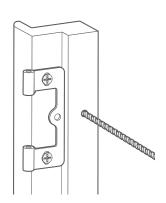
For 'Inside Recess' fitting, drill through the thicker section toward the back of the frame.
