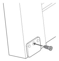
Finally, attach the metal strike plates to the back of the shutter panels, so that they're in line with the magnets.
