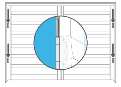
Now slot the hinge pins into place. Starting with the top hinge on each panel, align the panel part of the hinge with the frame part of the hinge, then insert the pin through the centre. If your shutter has folding panels, join these together the same way.
