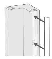
For Front of Recess frames, reinsert the decorative strips you removed in step 2.
