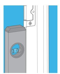
Make sure you also use the spirit level on the front of the frame, on all sides, to ensure there's no 'twist' to the frame.
