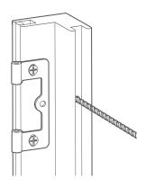
For "Front of Recess" fitting, remove the decorative strip covering the channel toward the back of the frame and drill your holes inside this channel.
