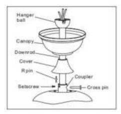
Loose the two setscrews in the downrod support.Return installing the Cross pin and secure with the R-pin.
