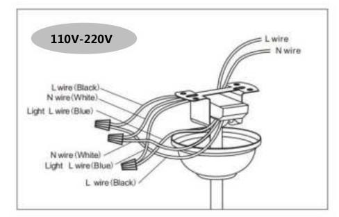
After wiring, attach the canopy to the hanger bracket by pushing up and twisting to locate screws in key holes then tighten screws securely.
