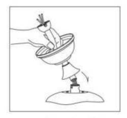
Remover the R-pin and Cross pin from downrod. Thread the wires through the downrod, and insert the Downrod into the Couple.
