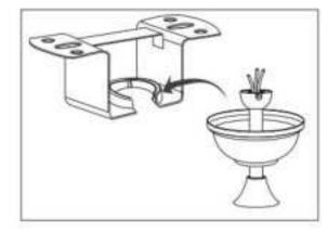
Carefully lift fan assembly into hanger bracket that is just attached to the outlet box. Be sure the groove in the ball is lined up with tab on the hanger bracket.
