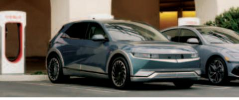
This Quick Reference Guide applies only to Tesla Superchargers. Tesla destination chargers at hotels or businesses, or home chargers are AC level 2 chargers.
