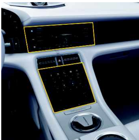
Fig. 5: Air-conditioning control panels
