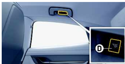
Fig. 93: Operating reading lights
