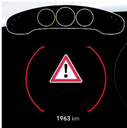
Fig. 219: Collision warning on the instrument cluster
