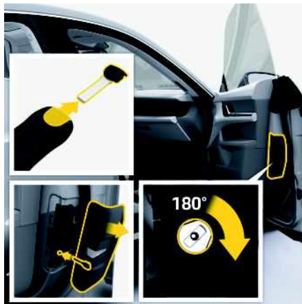
Fig. 44: Performing emergency locking of the passenger's door
