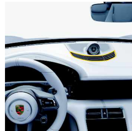
Fig. 21: Upper ventilation panel
