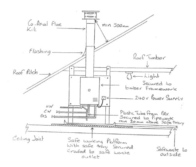
Note min height from working Platform to bottom of hot water unit > 500 mm
