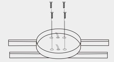
Self-tapping screw passes through the hanging plate hole then tighten it clockwise to lock the hanging plate.
