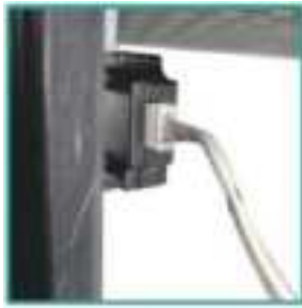
25. Plug the filament detection sensor cable
