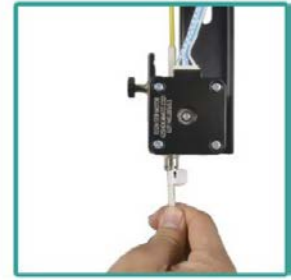
27. Push the PTFE tube to the position marked with an arrow in the photo
