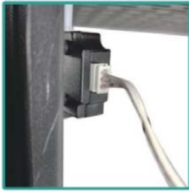
25. Plug the filament detection sensor cable
