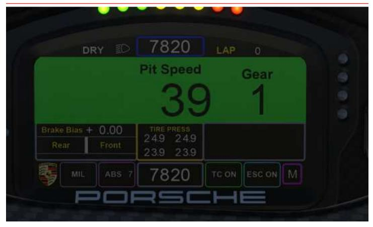
When the pit limiter is active a large green box containing the current speed and gear will fill the upper portion of the dashboard. The box will turn orange if traveling above the pit road speed limit with the limiter active.
