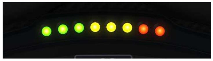
The shift lights illuminate from the outer edges inwardly. Illumination of the first LED will shift depending on the selected gear as such, the below values are only valid for 3rd gear.
