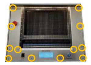
Remove the 14 screws from the front panels.
