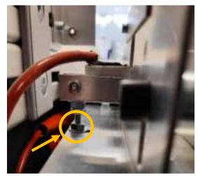
Adjust both height adjustment screws on both lamp holders. Adjust the lower nut and the one below the aluminum plate to perform this operation.
