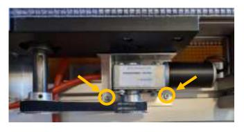
The motor belt tension is adjusted by two M4 screws that attach the motor assembly to the frame of the machine.
