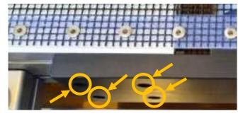
Release the four screws on both rear roller ends.
