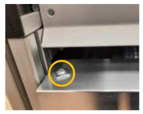
If needed, remove the rear paper collection plate, removing both screws.
