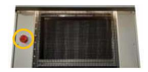
Remove the red mushroom button from the emergency stop switch, unscrewing it from the switch body.
