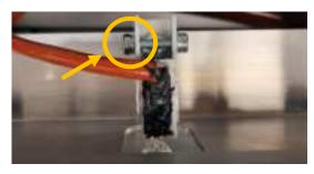
Release the M3 screws on both lamp holders. The lamp will come loose.
