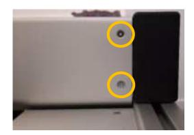
Remove the 8 screws from the top cover (front and back).
