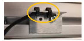
Temperature sensor #2: acquires the temperature of the external frame. This temperature is displayed in the LCD: "Te".
