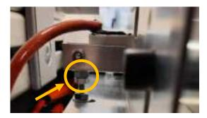
Make sure the two upper nuts are perfectly tightened.
