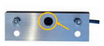
The belt rolling detector detects the correct rolling when the motor is "ON" and the lamp is "ON".
