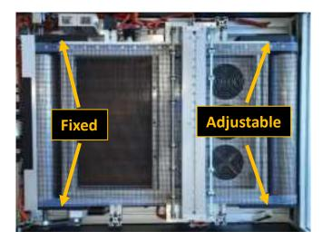
The two roller ends next to the paper exit are adjustable, allowing for paper belt tension adjustment.
