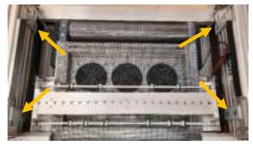
To ease the rest of the operation, it is recommended to remove the two upper lateral aluminum profiles, releasing the four tabs.
