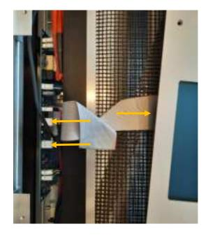
Gently remove the front lateral panels and the main front panel that contains the LCD display.
