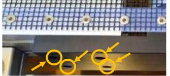
After the paper belt is properly adjusted, make sure to re-tighten all four screws on both roller ends.
