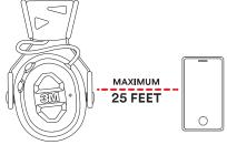
The typical range between a Bluetooth\* enabled device and the 3M Pro Electronic Hearing Protectors is approximately 25 feet. This distance may vary depending on the device. As the distance between the Bluetooth\* enabled device and the hearing protector increases, the risk of the signal dropping also increases.
