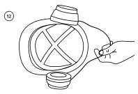
Remove the two suspension keys near the back of the hard hat (as shown in picture) by pulling them out of their key slots.
