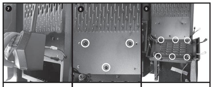
Disconnect two black and white wire connections on the side of the controller.
