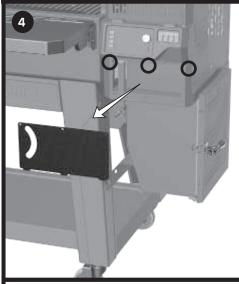
Remove 3 screws on the shutdown flap hopper shroud. Remove the shroud.
