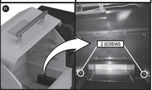
Remove the bottom (2 screws) next to the manifold inside of the body.
