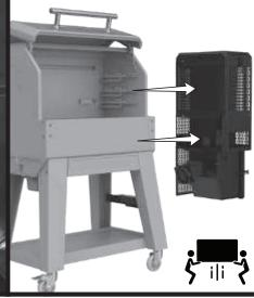
USE CAUTION, this step will disconnect the hopper from the body. Have a second party hold the hopper in place as your remove the hardware. Remove the top (2 screws) next to the manifold inside of the body. This will disconnect the hopper.
