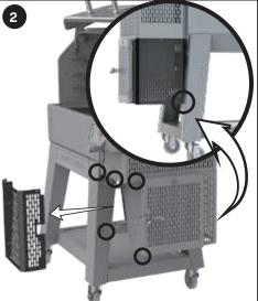
A) Remove the front hopper shroud.
