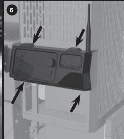
Remove the 4 thumb screws from the back of the controller. Remove the controller
