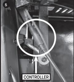
Remove the controller connections.
