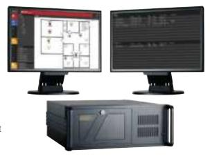
The gateway processes events and sends that information to a client using TCP/IP Ethernet protocol. The ONYXWorks client that receives and displays events for operators is the Workstation application. Since the gateway can reside on the same computer as the client, the information is simply transmitted from the gateway application to the workstation application over TCP/IP. To enable this communication, a computer IP address is required for all workstations and embedded gateways.
